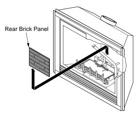
Figure 38 - Installing Rear Brick Panel
